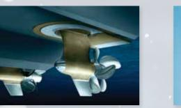
Zeus pods are independently steerable. The full force of each pod's thrust is directed independently to achieve much greater efficiency in manoeuvring.
