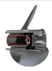
improvement vs. solid hub designs. The Flo-Torg SSR HD rotates both port and starboard - eliminating shift clunk and vibration for quiet and smooth shifting.
