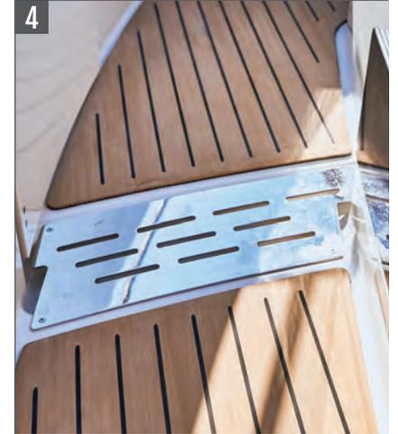
Drain system to avoid water accumulation
