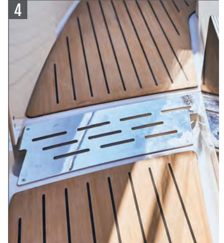
Drain system to avoid water accumulation
